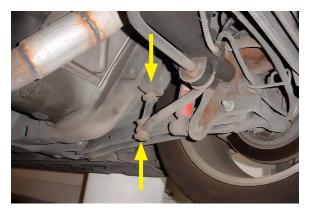
8. Remove the four 13mm nuts from the axle clamp to detach the sway bar and mounting brackets from the vehicle.
